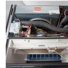
**HINGED DOOR TO PREVENT CONTAMINATION** Who knew hinges could be a sanitation feature? Unlike other manufacturers who require you to completely remove the front panel, the Indigo NXT has hinges, so you don't need to set it aside and risk exposure to contaminants when performing regular de-scaling and sanitizing.
